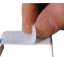
**STEP 6** Cut a piece of 'loop' Velcro to 4.5cm and attach as shown in figure to the right.
