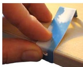
**STEP 5** Use a straight edge to fold the ends of the strip along the 18mm line from end of strip; leaving a 90 degree angle. In completing **STEP 7** adjust this angle to ensure there is minimal friction and to reduce side play.
