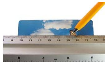
**STEP 2** On the 'back' side with the bar code, mark a line 18mm from each end.
