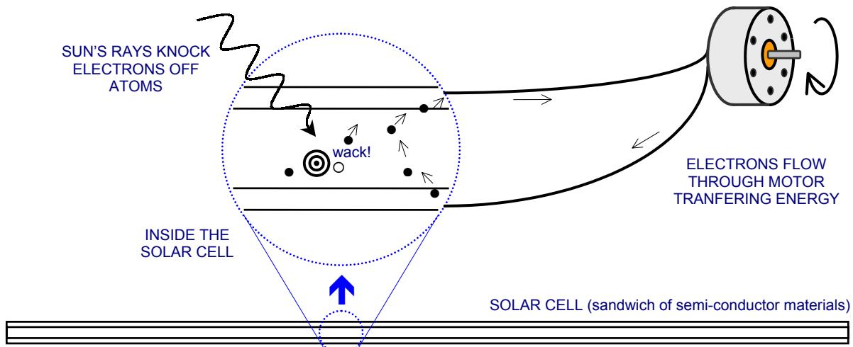
Now if we make an electric circuit with wires connecting the cell and a motor, electrons will flow through the motor (making it spin) and back to the solar cell where they can fill the "holes" left in the atoms which lost their electrons.
