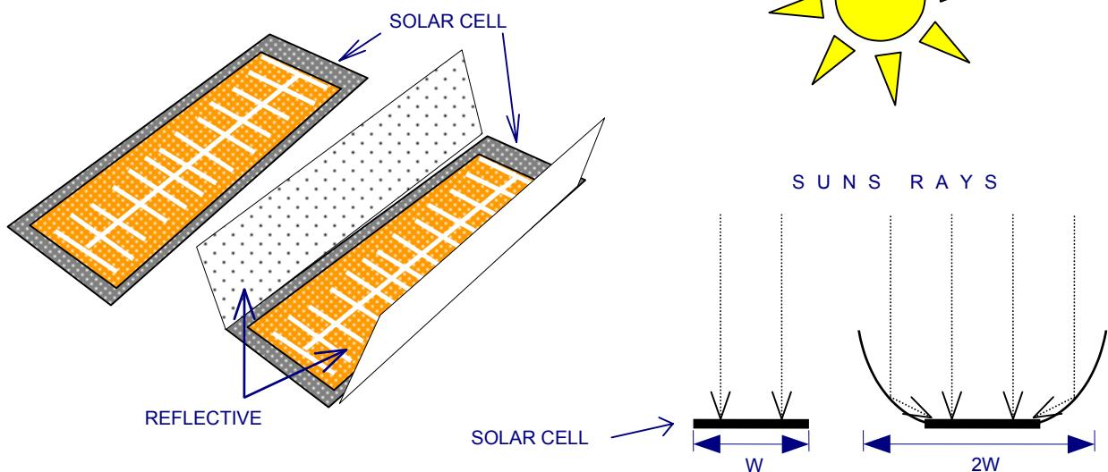
A reflector twice as wide as the solar cell can be made to capture twice as much sunlight.
