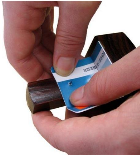
With the two curved edges of the card at the top and your thumbs on either side, carefully press the card onto the marking gauge. Ensuring the spike comes through in the middle of the card.
