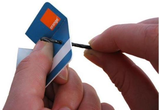
Using the 2mm drill bit, carefully twist through the hole made by the **scribe** removing all the swarf. You may need to repeat this process from the other side of the hole to ensure the axle can run freely. Repeat for other card.
