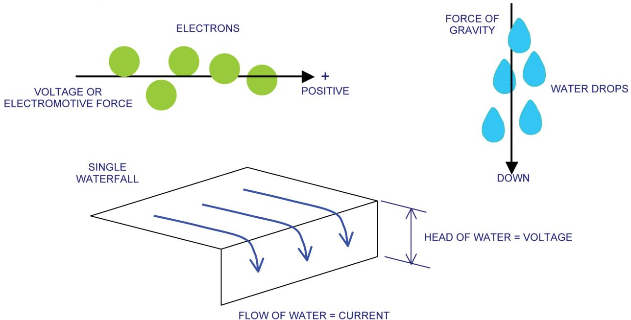
If we connect identical waterfalls in series and parallel it can help us see what happens when identical cells are connected in different ways.
