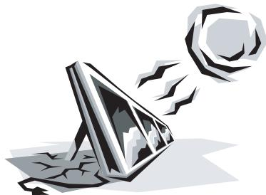
This ability results from the photovoltaic effect, a phenomenon in which the energy in sunlight causes electric charges to flow through layers of a conductive material to produce a useful electric current.
