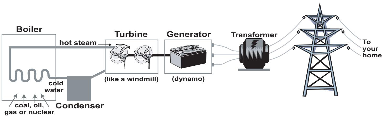
With a traditional power station energy sources such as coal, oil, gas or nuclear are transferred into electricity by a generator.
